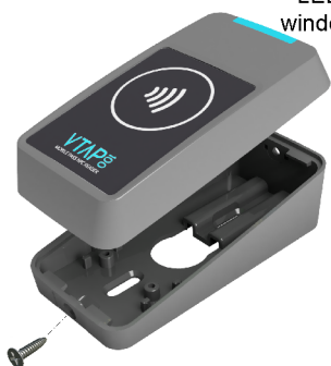
Figure 3-3 Wallmount or desktop assembly
