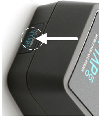
Figure 3-2 Where to apply pressure to slide label off case
