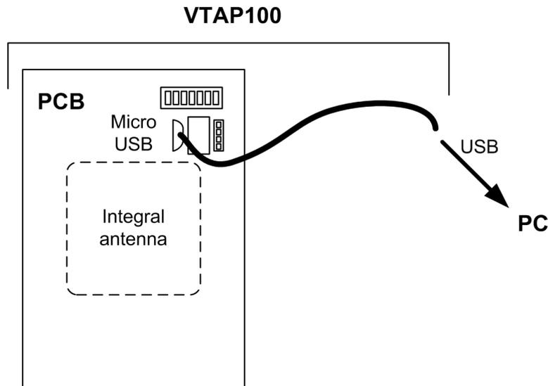
Figure 3-1 VTAP100 components - v4a or v5 Hardware
