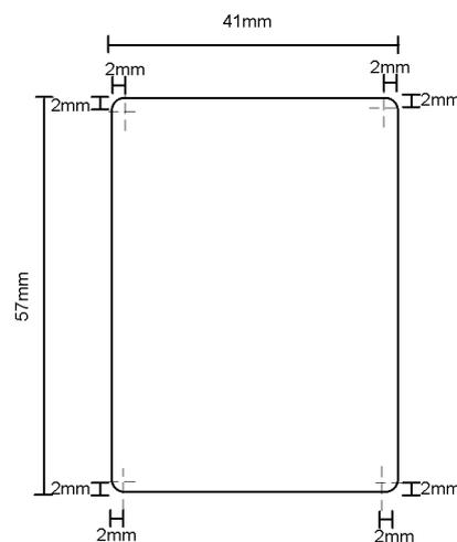
**Figure 3-6 Dimensions of label recess in -CC compact case**
