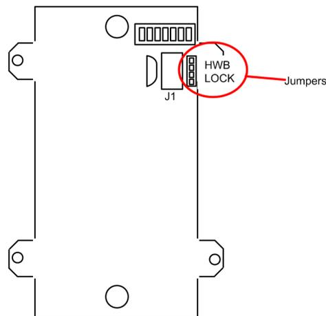
**Figure 5-1 Jumper positions on VTAP100 PCB v4a or v5 hardware**
