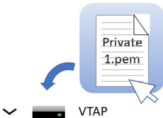
**Note:** When you reboot the VTAP100 your key will have been stored in hardware, and will no longer be listed as a file on the device. You can confirm key file(s) have been loaded when you **Check status in Boot.txt**. If the key file does not disappear and there is an error in `Boot.txt`, check your `.pem` file as it is likely it did not adhere to the standard - perhaps it was not an ECC key?
